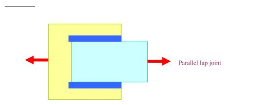
Figure 10.3.1: Different types of lap joints
